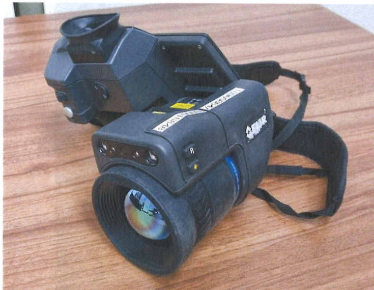
Figure 2. a) humidity and temperature meter, anemometer (wind speed meter); b) FLIR T1020 thermal imaging camera.
